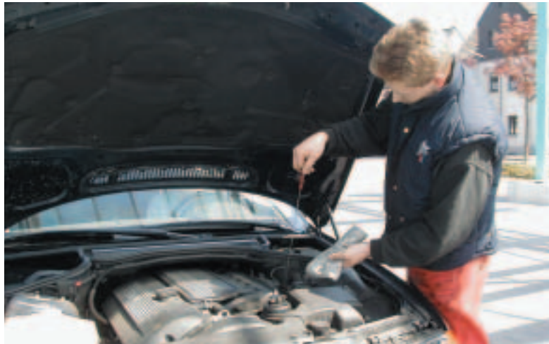
Oil level check using a dipstick
