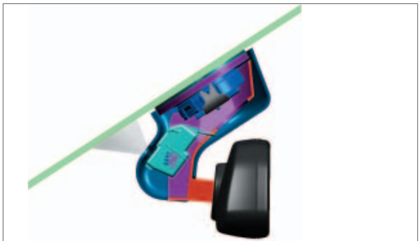
Cut through mirror base with integrated Thermopile sensor and Rain/Light sensor
